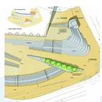
The scheme involved a complex design of gently graded ramps, integrated with tapering and sweeping curved steps and terraced seating steps, to deal with the significant level changes across the site. Materials used included York stone and Granite to complement the area's historic status adjacent to St. George's plateau.
